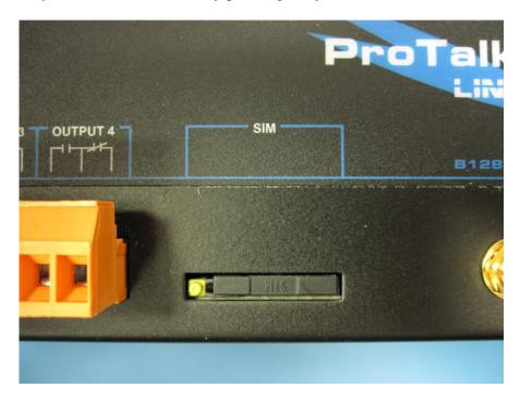
2) Remove the SIM card by pushing it out from the back of the holder with a narrow object. Insert the new card into the holder; making sure that it snaps into place.
