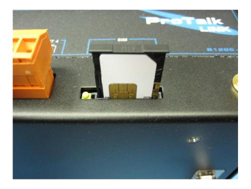
4) Apply power to the system and, using the configuration software, check to make sure that the MIN, ICCID and RSSI values are relevant. If the MIN number appears as ??????????, then the SIM card has not been activated:
